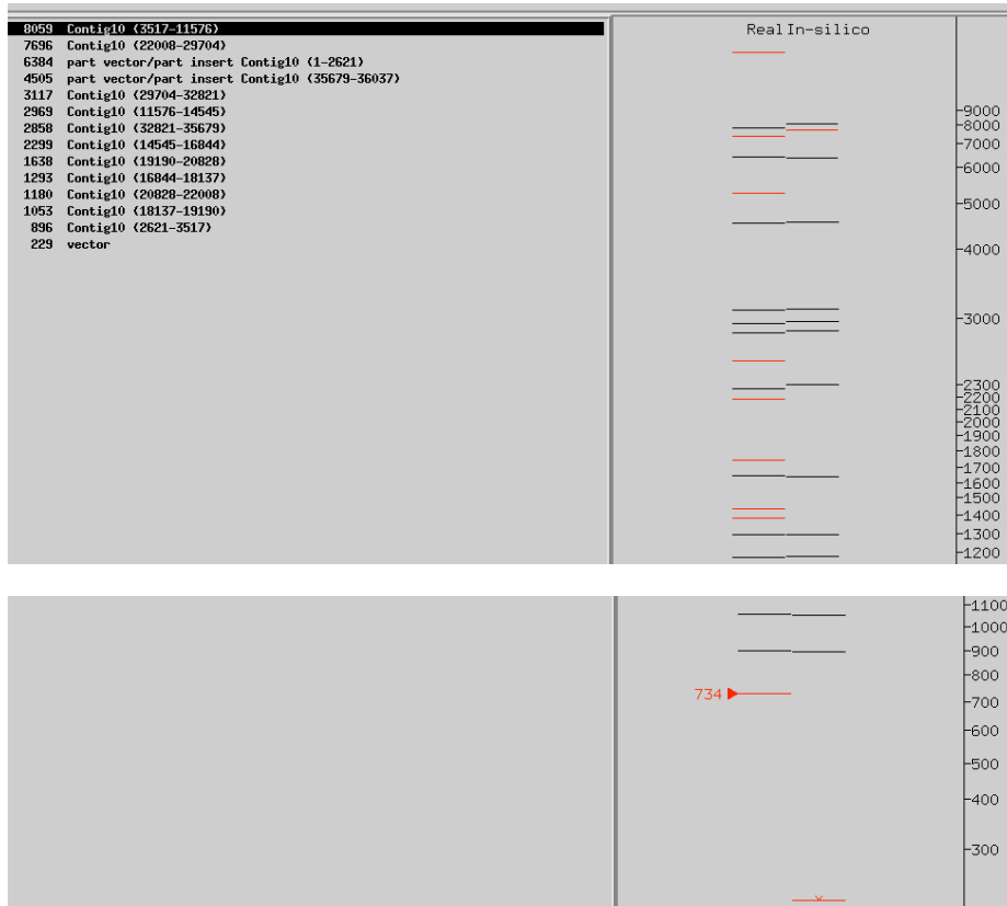
Fig. 10 Real vs. in silico EcoRI digest
